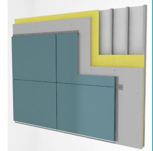
"Continuous Insulation is insulation that is uncompressed and continuous across all structural members without thermal bridges other than fasteners and service openings. It is installed on the interior or exterior or is integral to any opaque surface of the building envelope."
